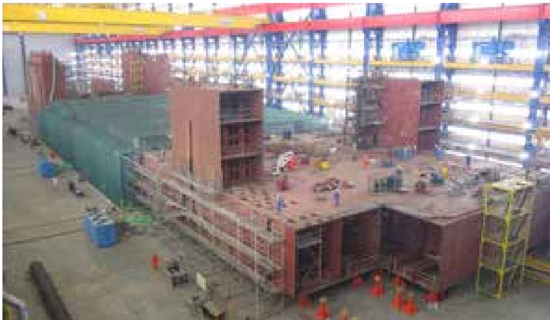
The 140m Load Out and Recovery (LOR) barge in build at NDSQ
