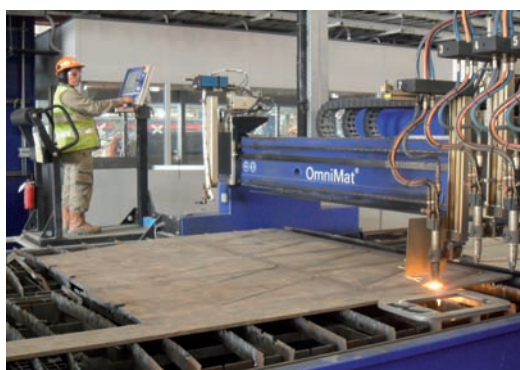
Cutting Steel and Fabrication of Dry Dock Gates
